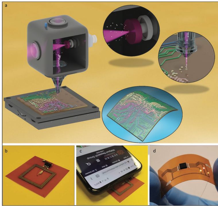
Figure 1. a) Schematic illustration of ANM process for dry printing Ag and ITO on flexible substrates. b,c) A 2 \times 2 \text{ cm}^2 printed Ag NFC tag antenna (four loops with a total length of \approx 32 \text{ cm} and \approx 1.38 \Omega \text{ cm} resistance) connected to a self-power M24LR04E IC enabling communication with a phone device. d) Printed FHEs circuit on the polyimide substrate.
